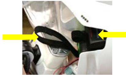
Battery handle on left; Battery inside the torso on the right Photos shown with torso skin removed for clarity
