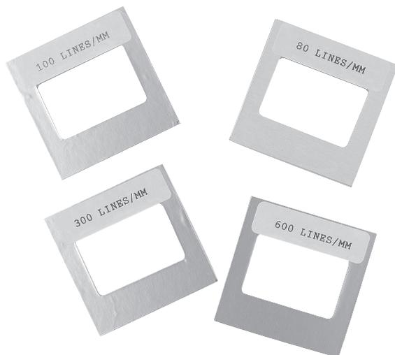
Transmission gratings for spectroscopic examinations and for experiments on diffraction and interference.
